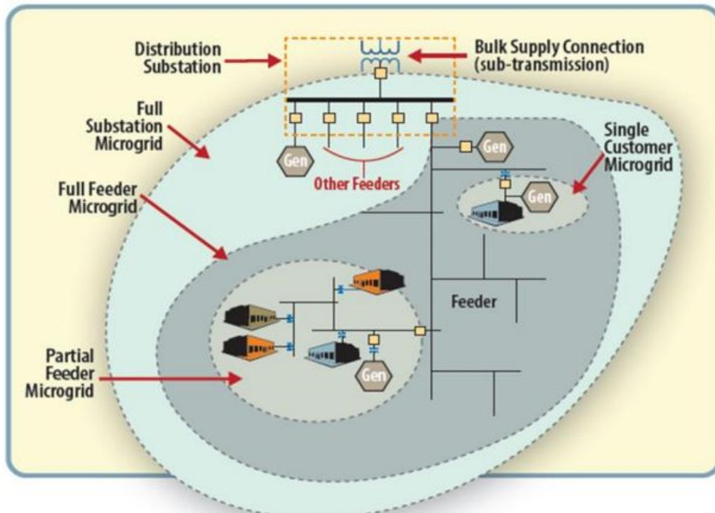
Figure 2: Board of Public Utilities (BPU) Microgrid Schematic
