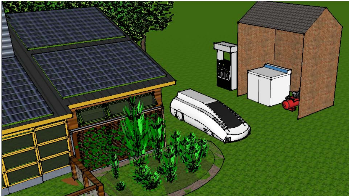
Figure 1.8: Hydrogen production unit for residential home. (Basic components are shown such as dispenser, electrolyzer, and compressor)
